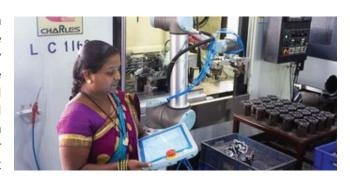
Shruthi Engineers realized the need for automation and installed the Cobots from Teradyne Robotics -UR10 to be used in CNC and Machine Tending tasks along with their existing workforce.
